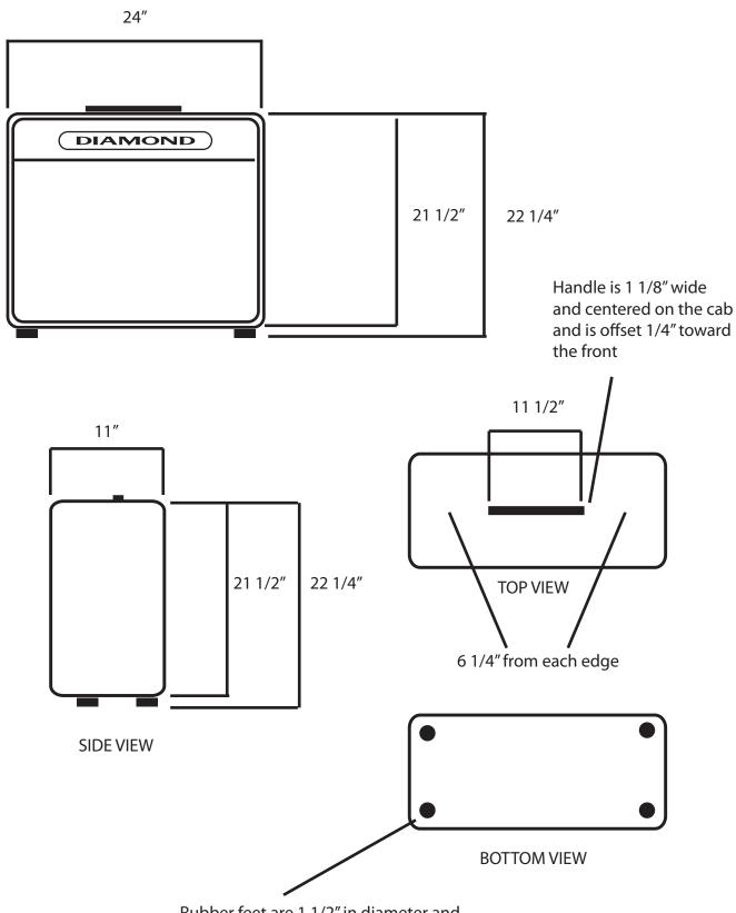
Rubber feet are 1 1/2" in diameter and are 1 1/4" from the nearest edges.
