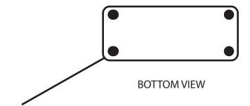
Rubber feet are 1 1/2" in diameter and are 1/2" from the outside edges, 1" from the front edge and 1/2" from the rear edge.
